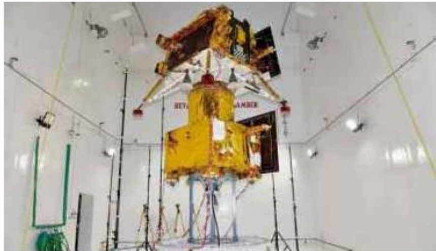
The Chandrayaan-3 propulsion module (top) attached to the lander (bottom) containing the rover, while undergoing a test. ISRO
